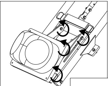
Loosen the screws that allow the platform to slide and tilt.
